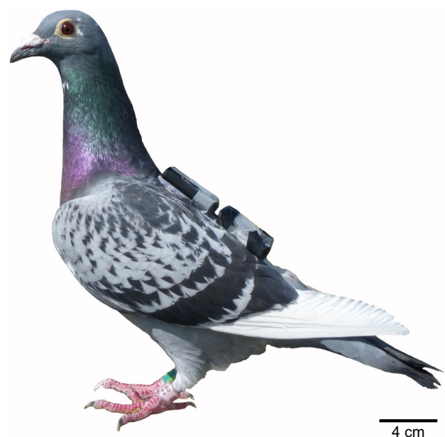
Fig. 1. A homing pigeon with an Axivity AX3 accelerometer (front) and Qstarz BT-Q1300ST GPS logger (case removed; back) attached to the back via Velcro strip, which was glued to trimmed feathers.
