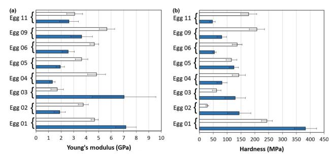
Figure 4. Nanoindentation measurements from eight eggshells laid by eight different female Greater Anis, showing (a) Young's modulus (GPa) and (b) hardness (MPa). Each bracket represents measurements from regions from the same egg presenting vaterite (open bars) or calcite (filled bars). [Colour figure can be viewed at http://onlinelibrary.wiley.com/journal/10.1111/(ISSN)1474-919X]
